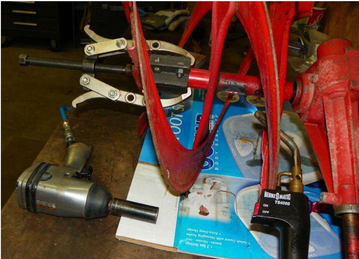
3. Drill a small hole in the center of the shaft. This will make the puller much more stable
